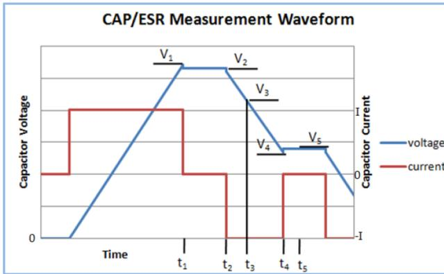
$$V1 = V_{\text{rated}} \quad t2 - t1 = 15 \text{ seconds} \quad \text{Capacitance} = I \times (t4 - t3) / (V3 - V4)$$
