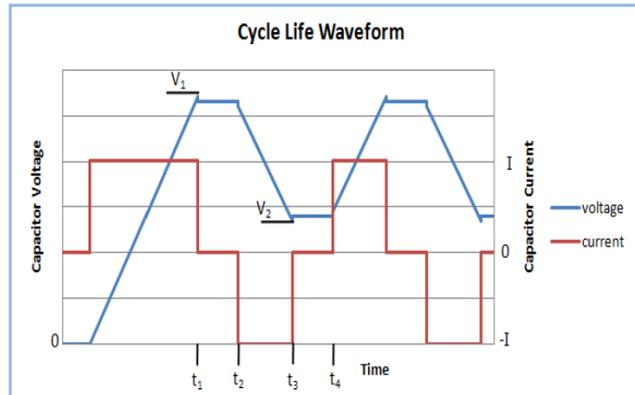
$$V1 = V_{\text{rated}} \quad t2 - t1 = 15 \text{ seconds}$$
